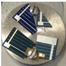
Figure 1. Photoconverter with pads
