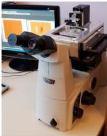
Installation for combined atomic-force and capillary microscopy on an inverted optical microscope Nikon Ti-U.
