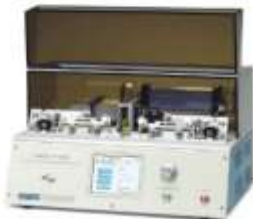
Puller P1000 (Sutter) for capillary pulling
