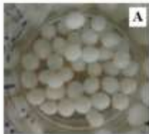
Fig. 10. Granules of HA / chitosan dispersed in an alkaline solution (A) and dried in air (B).
