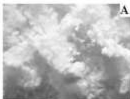
Photographs of a composite material with a filler content of 10%, A) t_{\text{drying}} = 200^{\circ}\text{C} , B) t_{\text{drying}} = 25^{\circ}\text{C}
