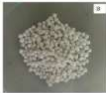
Fig. 11. Granules of brushite /chitosan dispersed in an alkaline solution (A) and dried in air (B).
